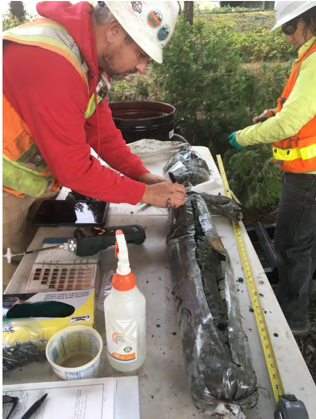
Soil sample to define contamination
